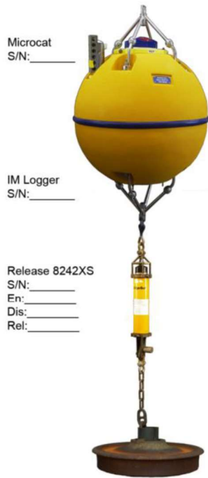
Figure 2. A photograph of the assembled COMIDA ADCP and MicroCat TCP mooring. The ADCP electronics are housed in the center well on the syntactic foam float. The MicroCat sits in a separate well with only the sensors exposed.
