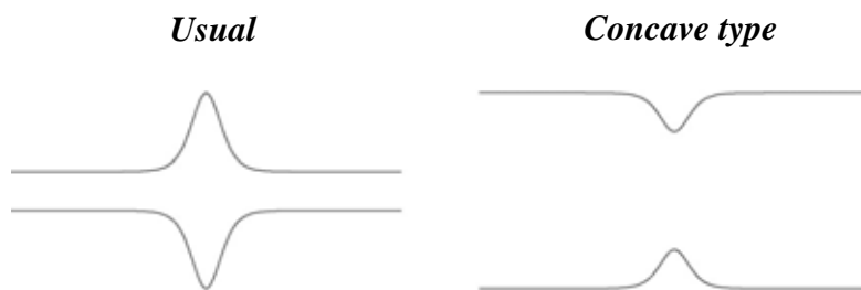
Fig.14 From left to right is the illustration of the mode-2 ISW (usual) and “concave type” mode-2 ISW.
